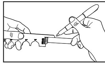
**4** Mark tube to proper fitting insertion depth with the Streamline® ACR Press Gauge or use the insertion depth chart below.
