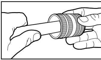
**2** Deburr tube ID & OD using a deburring tool. Ensure tube ends are free of any burrs or sharp edges.
