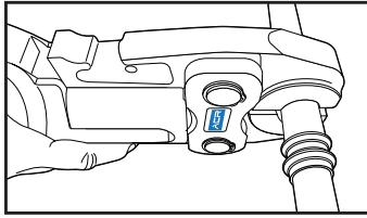
**7a** Place press jaw over both beads at a right angle to the tube. Start the pressing process. See tool manufacturer for tool instruction.
