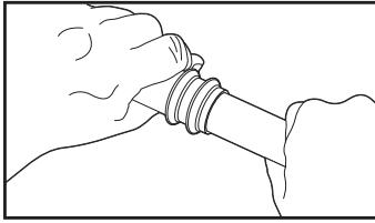
**6** Slightly rotate the fitting while sliding it onto tube. Slide all the way to insertion mark & make contact with stop.
