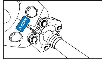
**7b** For 1-1/8"+ and all sizes Pivoting, use Streamline® ACR Press Ring, Ring Jaw, and compatible full-sized press tool. Place Press Ring over both beads at right angle to tube. Use ring jaw to start the pressing process.
