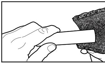
**3** Clean and smooth tube surface using a very fine abrasive pad. Tube surface should be free of indentation, scratches and deformations.
