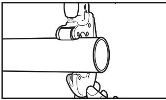
**1** Cut tube square using a tube cutter or fine tooth saw.
