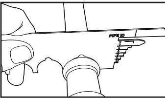
**8** Verify connection is secure using the Streamline® ACR Press Gauge between o-ring beads. Rotate gauge to avoid interference with flashing.
