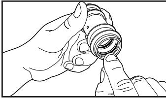
**5** Check both fitting beads to ensure two seals per cup are present.
